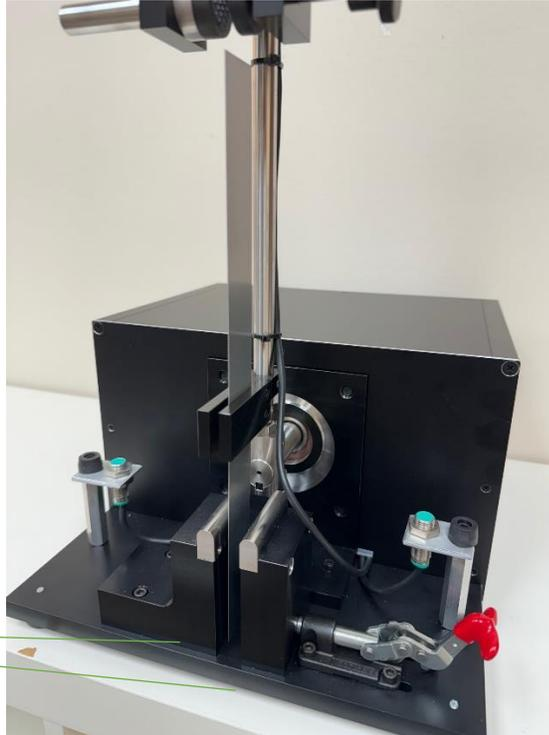
3. Push the red handle on the clamp forward to lock the sample into place.
