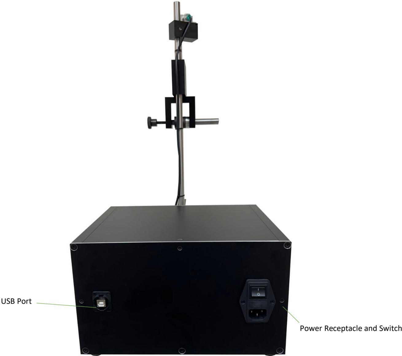
FIGURE 2-2 DUCTILITY TESTER CHASSIS FRONT OVERVIEW
